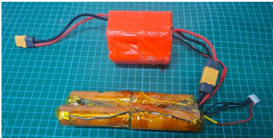
Figure 1. 3S4P custom-made battery pack for "Rico" UAV.
