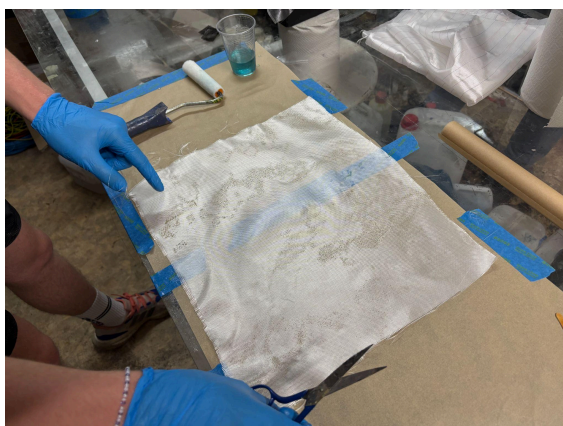
Fusing fiber with resin and placing it inside the mold.
