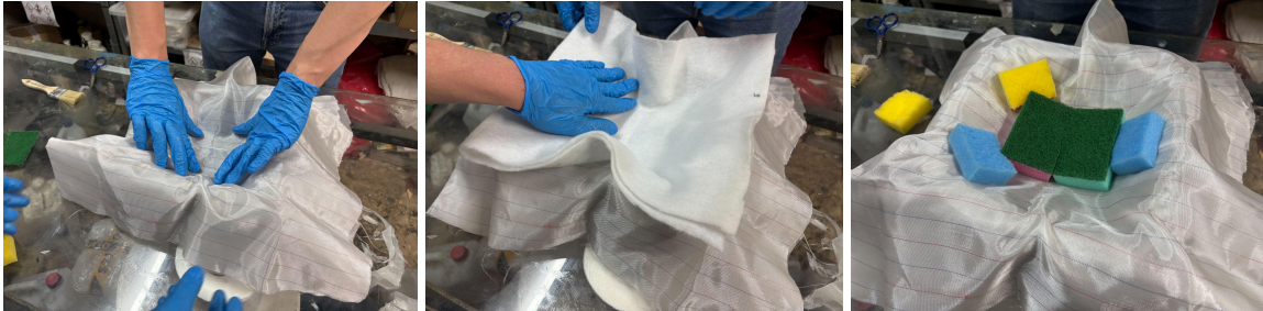
Placement of delamination insert, cloth and sponges.
